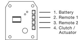
**REM 1** is intended for use when there is a need to allow a visitor to open the door after having been identified by intercom or by sight from within. REM 1 would be connected to a pushbutton on a reception desk, or to the appropriate button on an intercom. Pushing the button would cause the Blue LED to light and would release the lock for the normal set time.
