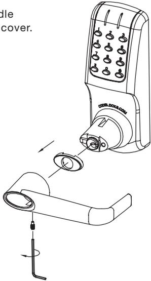
2. Turn key 90° clockwise and remove cylinder from boss.
