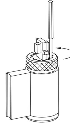
4. Replace the tailpiece, hold down the control pin and screw the cap fully on without tightening. Ensure control pin projects to lock the cap.
