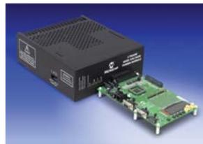
Power module shown with dsPICDEM MC1 Development Board (DM300020)
