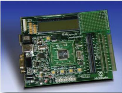
This development board offers an economical way to evaluate the PIC24F and PIC24H microcontrollers, the dsPIC33F General Purpose and Motor Control families and the PIC32 microcontroller families. This board is an ideal prototyping tool to help you quickly develop and validate key design requirements.
