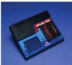
MPLAB PM3 Device Programmer is a full-featured, production quality universal device programmer. Using interchangeable socket modules, the MPLAB PM3 supports virtually all programmable devices from Microchip. MPLAB PM3 has improved programming time for many devices and offers a built-in interface for robust ICSP.
