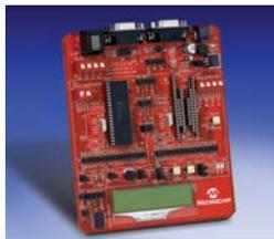
This development board provides a cost effective way to start designing solutions for all 18-, 28- and 40-pin DIP-packaged dsPIC DSC devices.
