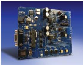
This development board implements a simple DC/DC Switch Mode Power Supply (SMPS) and is a good starting point for designers new to digital loop control design.
