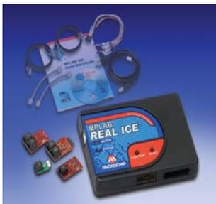
The MPLAB REAL ICE In-Circuit Emulator is Microchip's next-generation emulation and debugging system. Initially supporting the dsPIC33F, PIC24H, PIC24F and dsPIC30F601XA 16-bit devices, this system provides a powerful in-circuit emulation platform for easy and rapid application development
