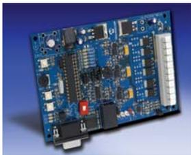
This board provides a cost-effective method of evaluating and developing sensed or sensorless BLDC motor control applications. A 28-pin, dsPIC30F3010 device is used with this board.
