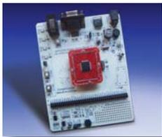
This development board offers a very economical way to evaluate the 80-pin dsPIC30F General Purpose and Motor Control families as well as the dsPIC33F devices.
