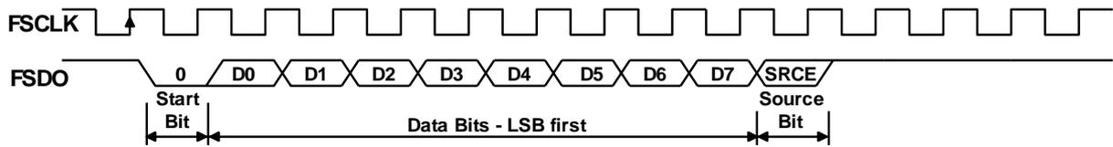
**Figure 4.14 Fast Opto-Isolated Serial Interface Output Data**
