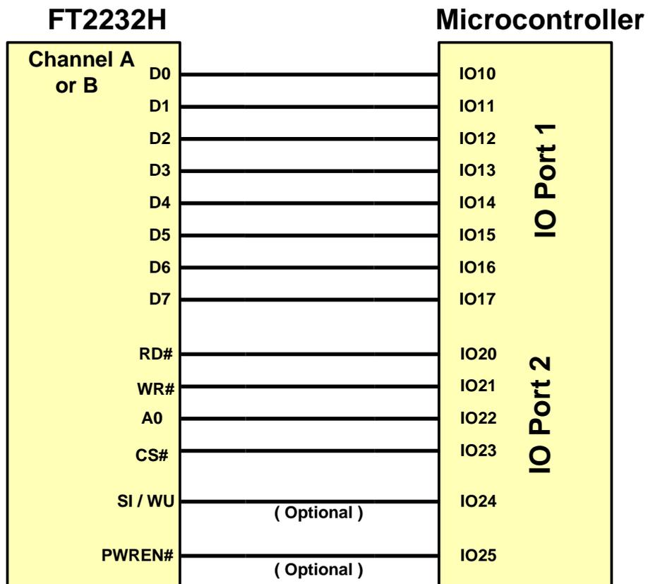
**Figure 4.18 CPU-Style FIFO Interface Example**
