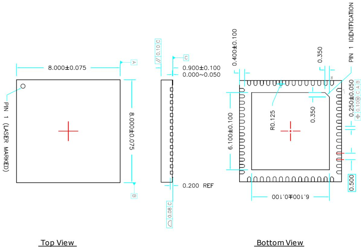
Figure 8.3 56-pin VQFN Package Details for FT2232H-56Q
