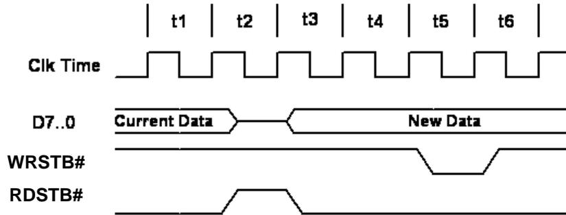
**Figure 4.19 Synchronous Bit-Bang Mode Timing Interface Example**
