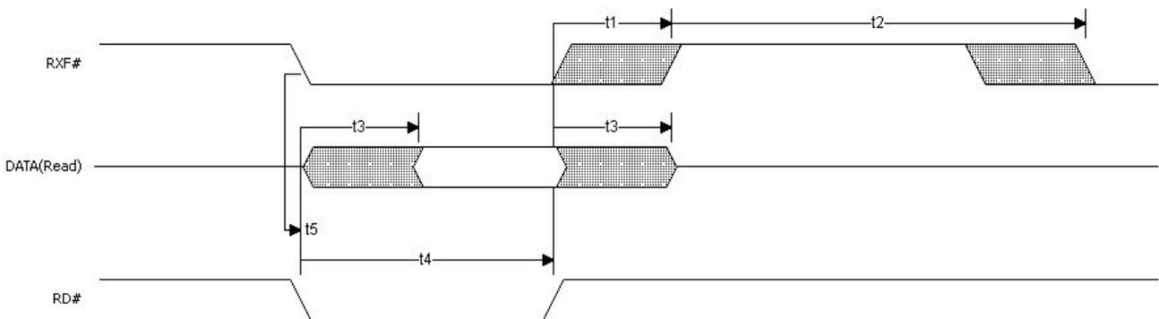
**Figure 4.5 FT245 asynchronous FIFO Interface READ Signal Waveforms**
