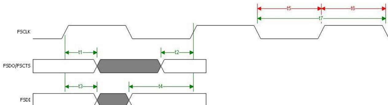
**Figure 4.13 Fast Opto-Isolated Serial Interface Signal Waveforms**
