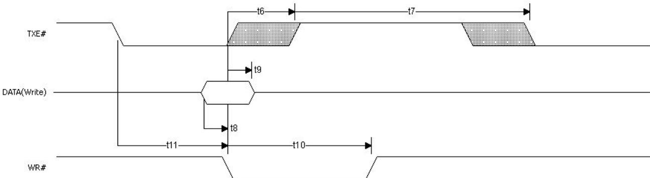
**Figure 4.6 FT245 asynchronous FIFO Interface WRITE Signal Waveforms**
