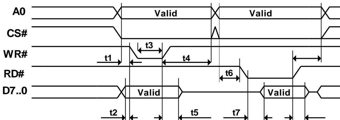
**Figure 4.17 CPU-Style FIFO Interface Operation Signal Waveforms.**
