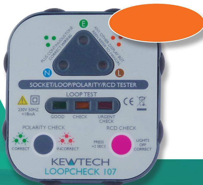
The loopcheck 107 also has the ability to check for the correct polarity of the mains supply. If this is wrong then a very hazardous situation exists. By touching the left hand touch pad the correct polarity of the mains supply is verified. The right-hand test button puts out a measured tripping current to check the operation of 30mA RCDs.
