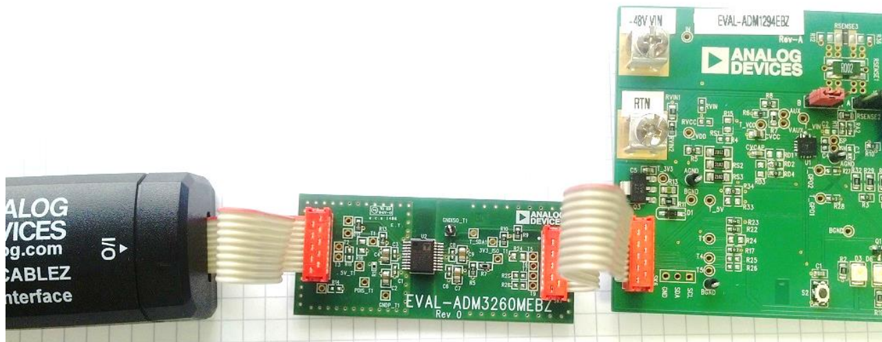
Figure 2. Board Connection Example
