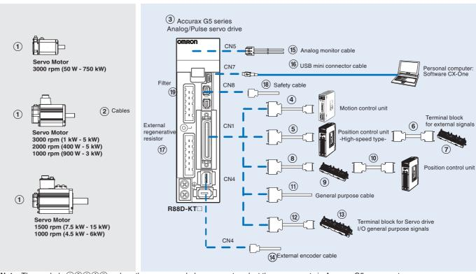
Note: The symbols ① 2 3 4 5 ... show the recommended sequence to select the components in Accurax G5 servo system
