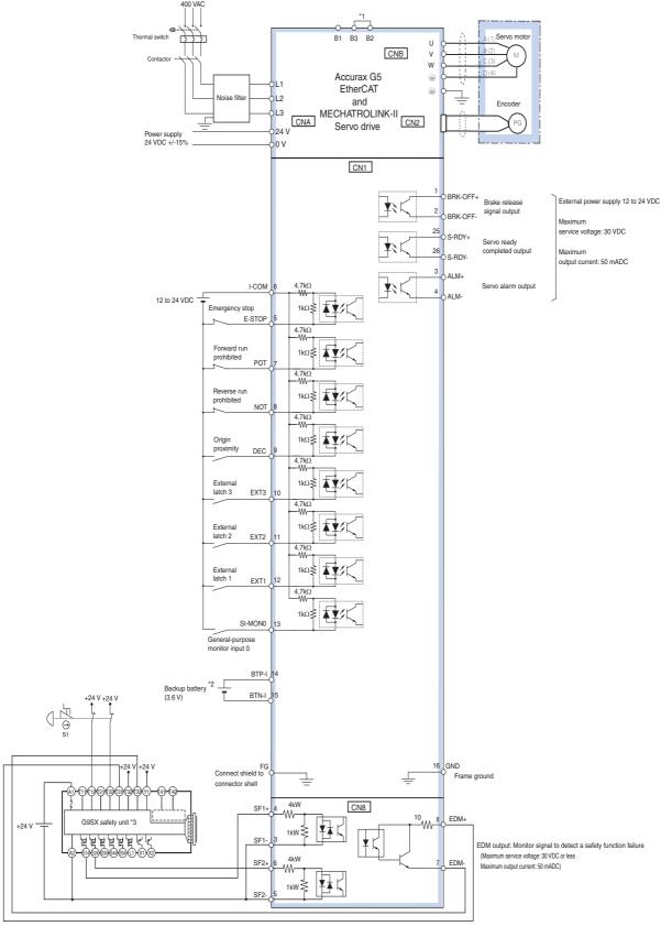
Normally B2 and B3 are short-circuited. If the internal regenerative resistor is insufficient, remove the wire between B2 and B3 and connect an external regenerative resistor between B1 and B2.
