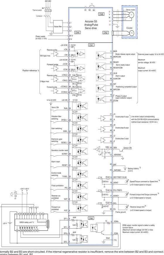
Normally B2 and B3 are short-circuited. If the internal regenerative resistor is insufficient, remove the wire between B2 and B3 and connect an external regenerative resistor between B1 and B2.
