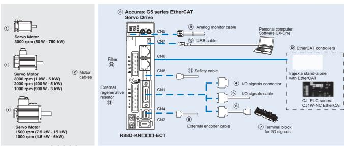
Note: The symbols (12345)... show the recommended sequence to select the components in Accurax G5 servo system
