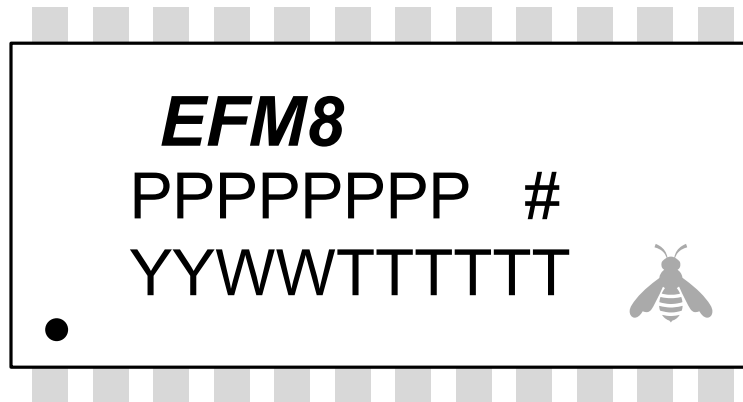
Figure 10.3. QSOP24 Package Marking
