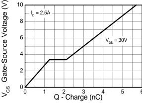
**Gate-Source Voltage v Gate Charge**
