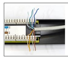
2) Untwist the pairs and place the wires on the IDC block in the correct configuration for either T568A or T568B.
