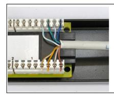
4) If the punch down tool does not cut excess wire, trim the excess wire off.
