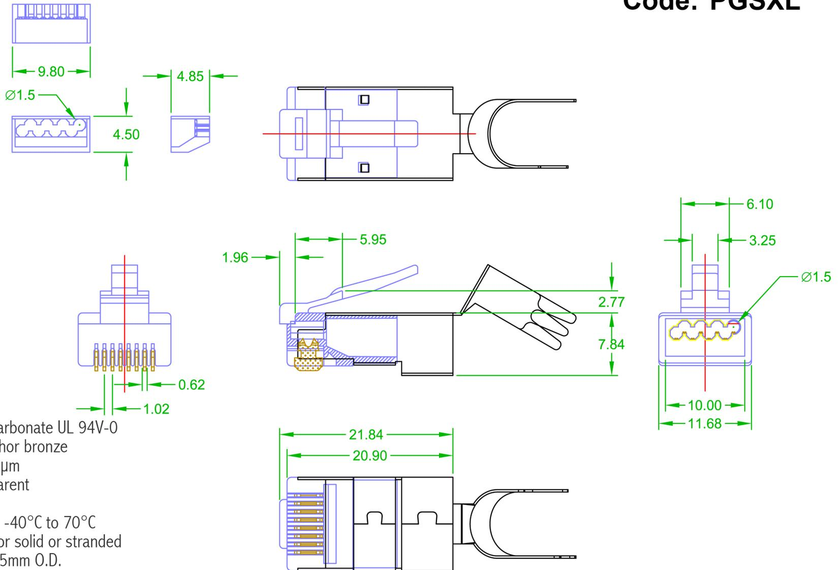
1. Housing Material: Polycarbonate UL 94V-0
