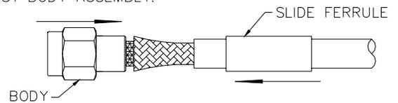
8. CRIMP OUTER FERRULE WITH APPROPRIATE CRIMP TOOL.
