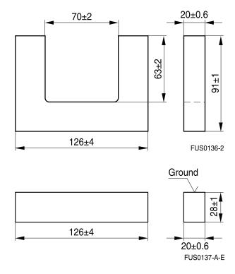
U and I cores are supplied as single units. The  $A_L$  value in the table applies to a core set comprising two ungapped cores.
