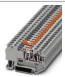
Knife disconnect terminal block, Connection type: Spring-cage connection, Cross section: 0.08 mm² - 6 mm², AWG: 28 - 10, Nominal current: 20 A, Nominal voltage: 400 V, Length: 61.5 mm, Width: 6.2 mm, Color: gray, Assembly: NS 35/7,5, NS 35/15
