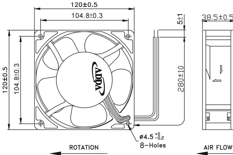
LEAD WIRES : UL 1007, AWG24 , L = 280±10 mm
