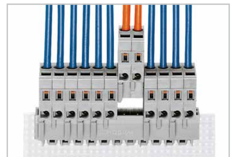
Female connectors with built-in end plate require no extra space, while maintaining the nominal cross-section. This means: Total length of female connectors is reduced to "pole no. x pin spacing"!
