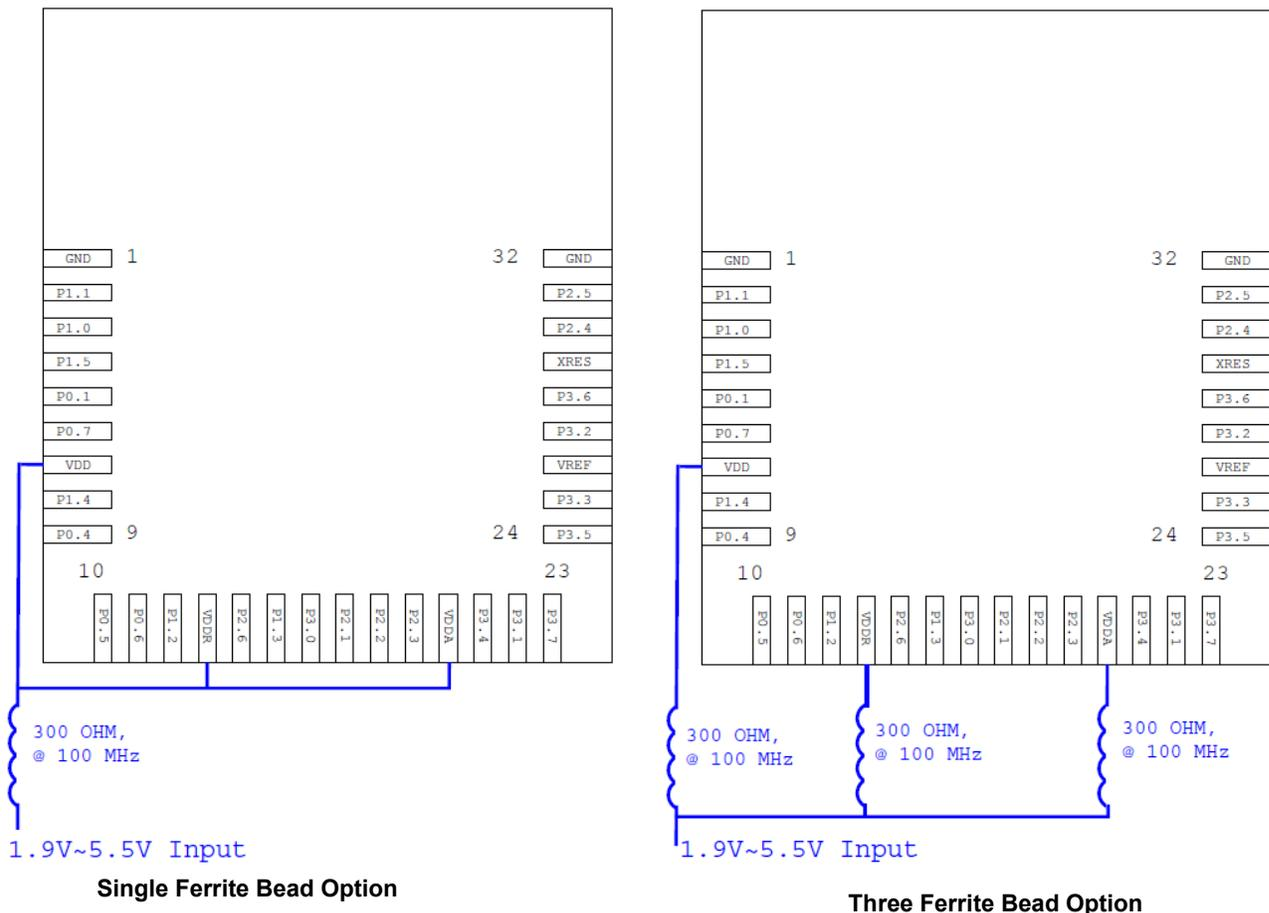
Figure 8. Recommended Host Schematic for Independent Supply Option
