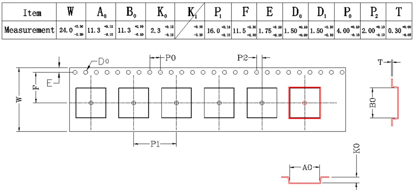
[Figure 11](#) details the orientation of the CYBLE-014008-00 in the tape as well as the direction for unreeling.
