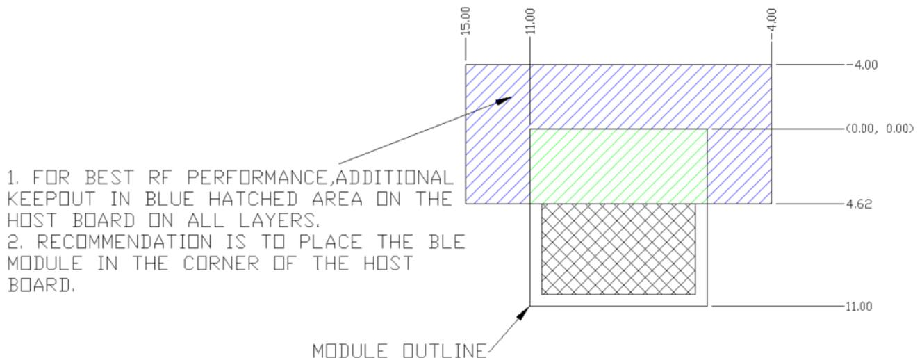
1. FOR BEST RF PERFORMANCE, ADDITIONAL KEEPOUT IN BLUE HATCHED AREA ON THE HOST BOARD ON ALL LAYERS.
