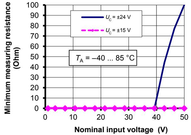
Figure 2: Minimum measuring resistance.
