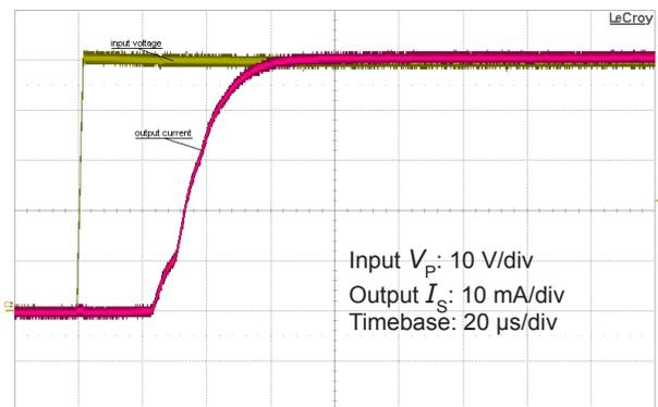
Figure 6: Typical step response (0 to 50 V)
