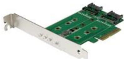
This 3-port M.2 SSD adapter card is one of the only cards that supports both PCIe and SATA-based M.2 SSDs (solid-state drives). It's a versatile way to expand the overall storage capacity of your desktop PC or server. Plus, because it supports a high-speed PCIe M.2 drive, you can increase the speed and performance of your computer.
