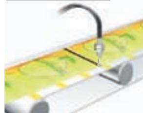
In Black Mode, blank seam tape and other black marks can be detected regardless of film color or patterns
