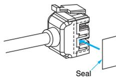
Note: Attach the seals to the sides with grooves.
