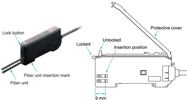
Note: Do not pull on, compress, or otherwise exert excessive force on the fiber units after connecting them to the Amplifier Unit.
