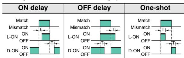
2. Control Outputs (AND, OR, Sync) and Timing Chart for Timer Settings (T: Set Time)
