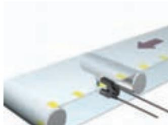
Through-beam heads are capable of detecting color differences in semi-transparent objects.
