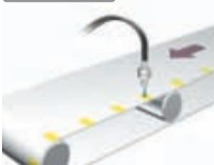
Because it distinguishes RGB ratios, detection is highly resistant to workpiece movement.
