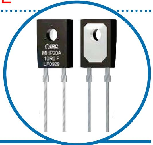
IRC's MHP20S series resistors satisfy demanding applications for accurate and stable power resistors housed in the convenient TO-126 case. The resistance element is isolated from the mounting tab by an alumina ceramic layer, providing very low thermal resistance and ensuring high insulation resistance between terminals and tab. The non-inductive design makes these products especially useful in high frequency and high speed pulse applications.
