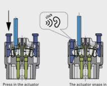
Press in the actuator using gentle finger pressure.
