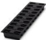
Header, Nominal current: 12 A, Rated voltage (III/2): 320 V, Number of positions: 6, Pitch: 5.08 mm, Color: black, Contact surface: Tin, Mounting: THR soldering, User information and design recommendations for through hole reflow technology can be found under "Downloads"
