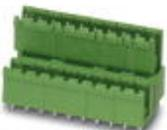
Header, Nominal current: 10 A, Rated voltage (III/2): 320 V, Number of positions: 6, Pitch: 5.08 mm, Color: green, Contact surface: Tin, Mounting: Wave soldering, Can be aligned! Mounting flange: Order No. 1836477, 1836480. In combination with MVSTB or FKCV plug components, both an MVSTBW (or FKCVW) and an MVSTBR plug (or FKCVR) must be used. Combination with TMSTBP plug components is not possible!
