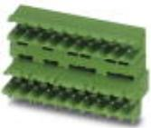
Header, Nominal current: 10 A, Rated voltage (III/2): 320 V, Number of positions: 6, Pitch: 5.08 mm, Color: green, Contact surface: Tin, Mounting: Wave soldering, The article can be aligned to create different nos. of positions! In combination with MVSTB or FKCV plug components, both an MVSTBW (or FKCVW) and an MVSTBR plug (or FKCVR) must be used. Combination with TMSTBP plug components is not possible!
