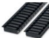
Header, Nominal current: 12 A, Rated voltage (III/2): 320 V, Number of positions: 6, Pitch: 5.08 mm, Color: black, Contact surface: Tin, Mounting: THR soldering, Two-in-one – Pin strips must always be made up of a left (L) and a right (R) segment. Please allow for the corresponding counterpart from the accessories to complete the THR pin strip.
