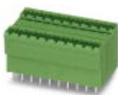
Header, Nominal current: 10 A, Rated voltage (III/2): 320 V, Number of positions: 6, Pitch: 5.08 mm, Color: green, Contact surface: Tin, Mounting: Wave soldering, In combination with MVSTB or FKCV plug components, both an MVSTBW (or FKCVW) and an MVSTBR plug (or FKCVR) must be used. Combination with TMSTBP plug components is not possible!
