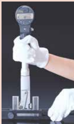
Origin setup gage block set
