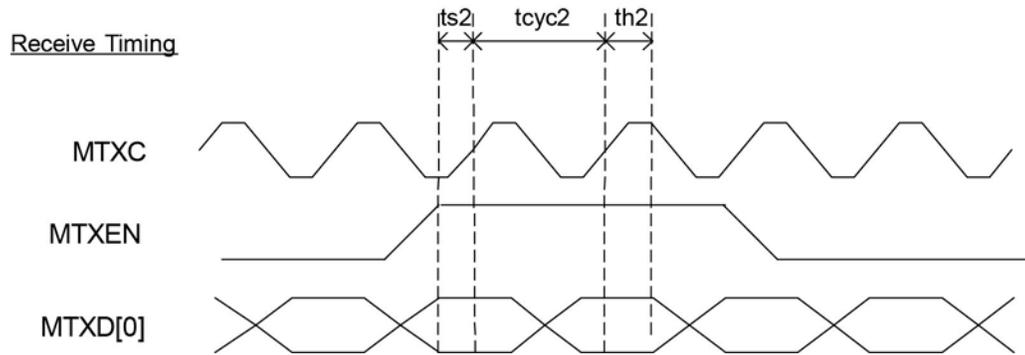
**Figure 21. SNI Input Timing**
