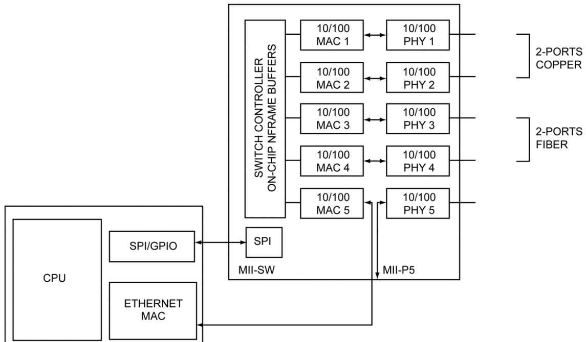
Figure 4. Using KSZ8895FQX for Dual Media Converter
