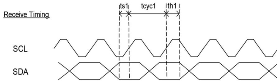
Figure 19. EEPROM Interface Input Receive Timing Diagram
