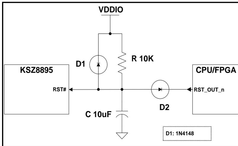
**Figure 35. Recommended Circuit for Interfacing with CPU/FPGA Reset**
