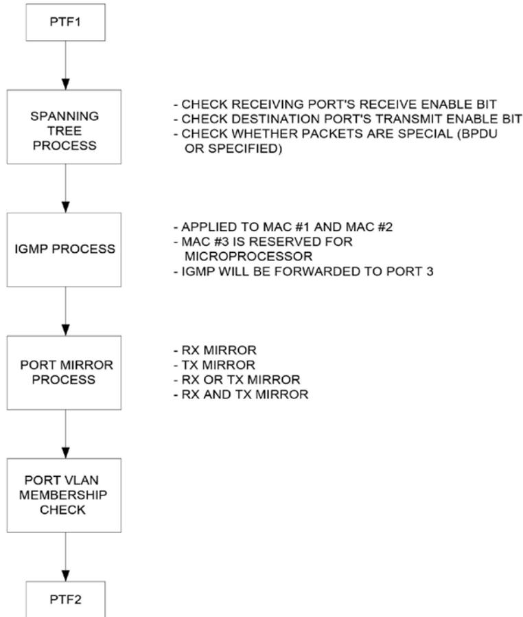
**Figure 11. Destination Address Resolution Flow Chart, Stage 2**
