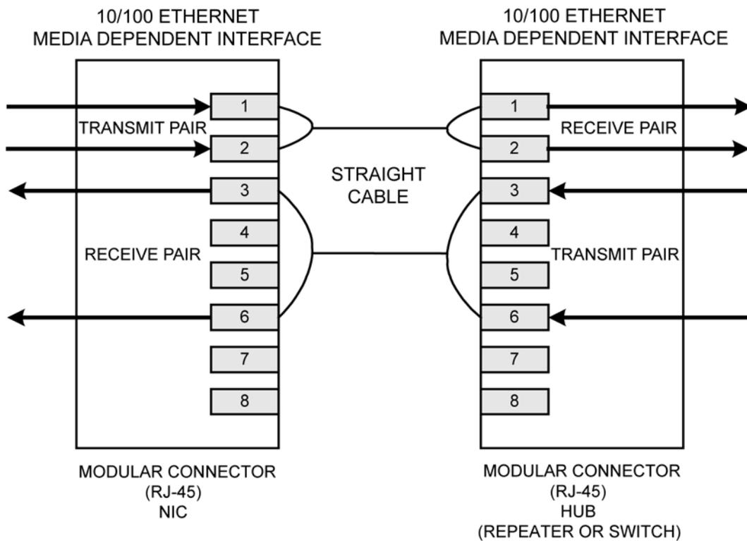
**Figure 5. Typical Straight Cable Connection**
