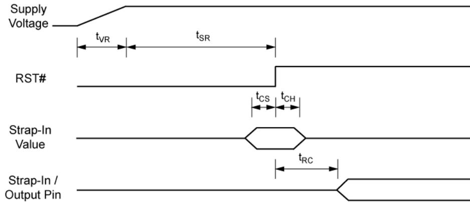
**Figure 33. Reset Timing**
