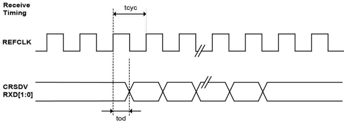
**Figure 28. RMII Timing – Data Transmitted to RMII**
