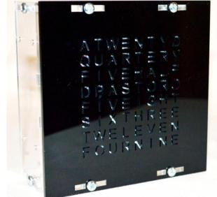
The front plate is interchangeable to allow the assembly to be used for different purposes such as pixel art, games or displaying information.
