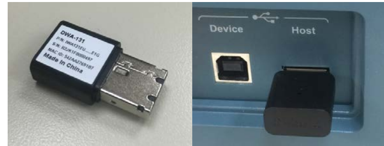
Figure 18. Insert the TEK-USB-WIFI adapter to enable wireless communications
