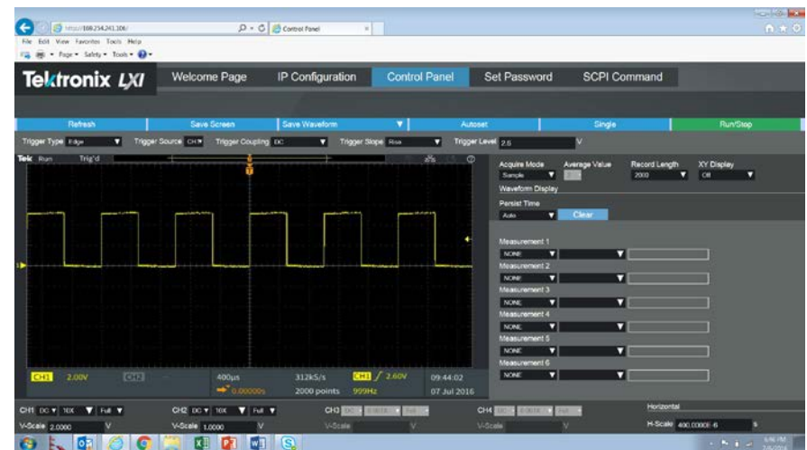
Figure 21. On the PC, the IP has been entered into the address box of the browser, and autoset has been performed remotely
