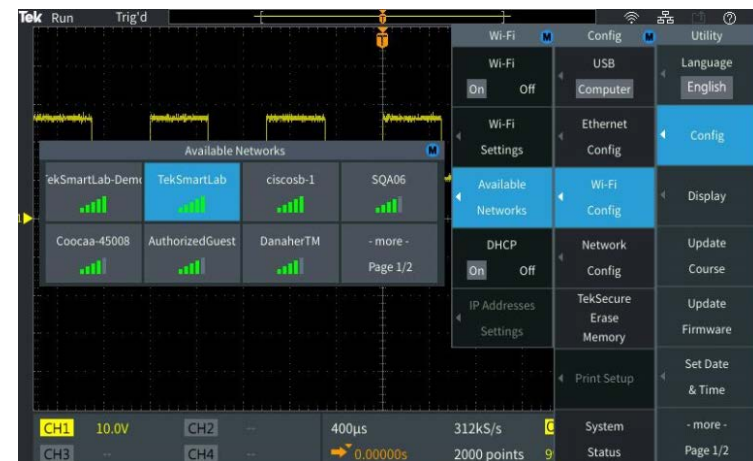
Figure 19. Configuring Wi-Fi communications via the Utility Menus
