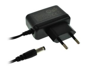
This switch mode power supply is rated to 6W maximum, providing a regulated 12vdc output at up to 0.5A with no minimum load. The unit meets Level V efficiency standards. This power supply carries full safety approvals. Short circuit and over current protection is integral.
