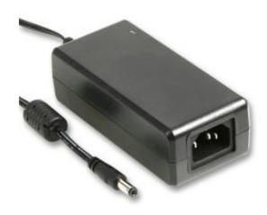
This switch mode power supply is rated to 50W maximum, providing a regulated 15vdc output at up to 3.34A with no minimum load. The unit meets latest CoC Tier 1 / Level VI efficiency standards and will be uprated to CoC Tier 2 requirements before the requirement is made mandatory. This power supply carries full safety approvals. Short circuit and over current protection is integral.
