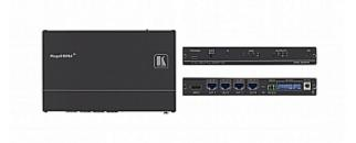
The VM-4HDT is a high-quality 1:4 4K UHD HDMI to HDBT distribution amplifier that takes one HDMI input, equalizes and reclocks the signal and distributes it to four identical HDBT outputs. The VM-4HDT distributes signals having resolutions of up to 4K@60Hz (4:2:0) UHD including WUXGA and 1080p.
