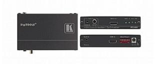
The FC-69 is a high-performance 4K@60Hz (4:2:0) UHD, 4Kx2K HDMI audio embedder and de-embedder. The unit can embed analog audio to the HDMI output or de-embed audio from the HDMI input or from the HDMI output Audio Return Channel to S/PDIF and unbalanced stereo audio outputs simultaneously.
