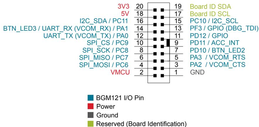
Figure 4.3. Expansion Header
