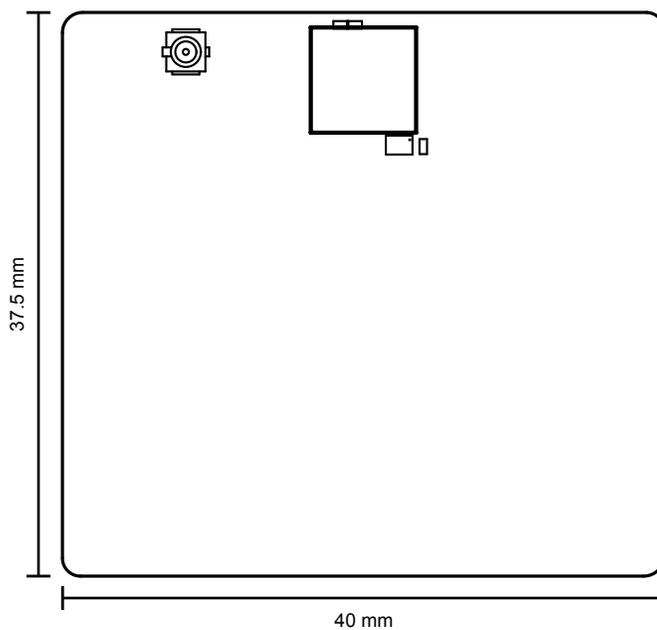
Figure 14.1. BRD4302A Top View
