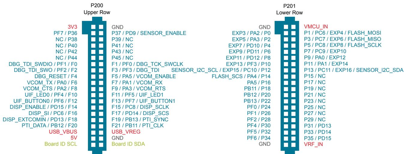
Figure 13.1. Radio Board Connectors
