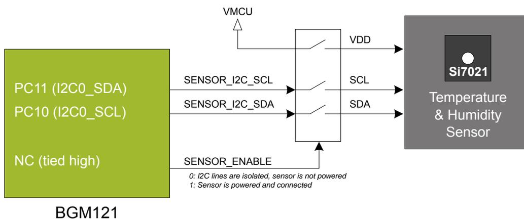
Figure 6.4. Si7021 Relative Humidity and Temperature Sensor
