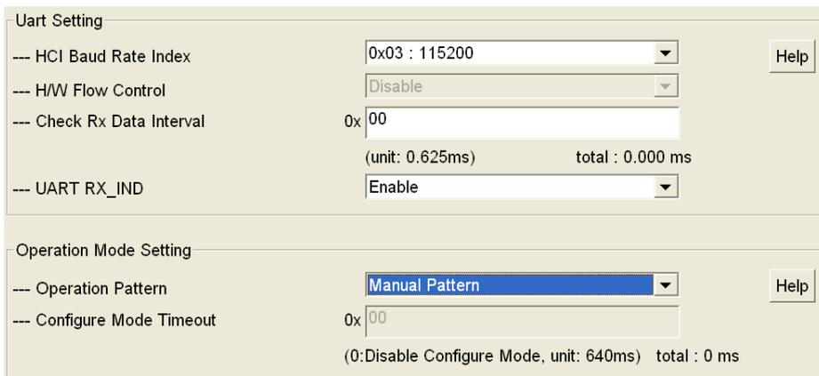
ii. UI Tool: in system setup2 page, configure the GPIO vs function mapping. In manual pattern tool, only RX\_IND configuration is valid.
