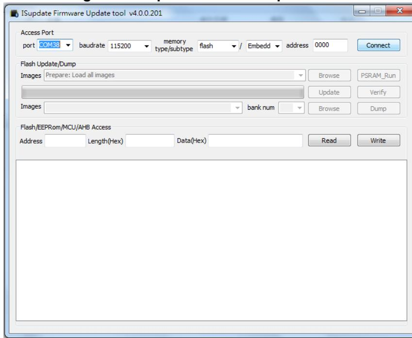
**Note:** Verify BLEDK3 device features in the “Release Note” Document. If an update to newer firmware version is necessary, then the flash code should be downloaded first, before the UI parameters are loaded. As the flash update process could overwrite the UI parameter configuration.
