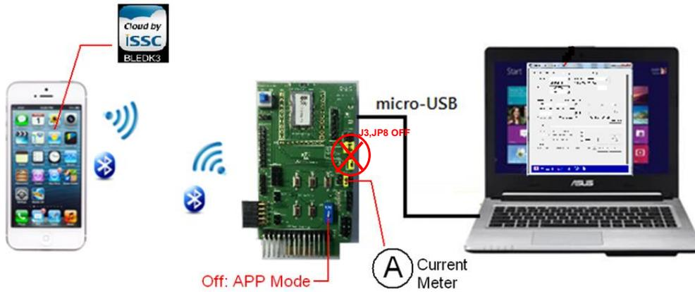
**- BLEDK3 APP Setup:** Make link and click to transparent page to test current in connected mode
