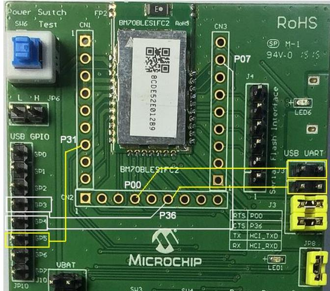
d. In this example, the mapping table between module and USB GPIO is as below:
