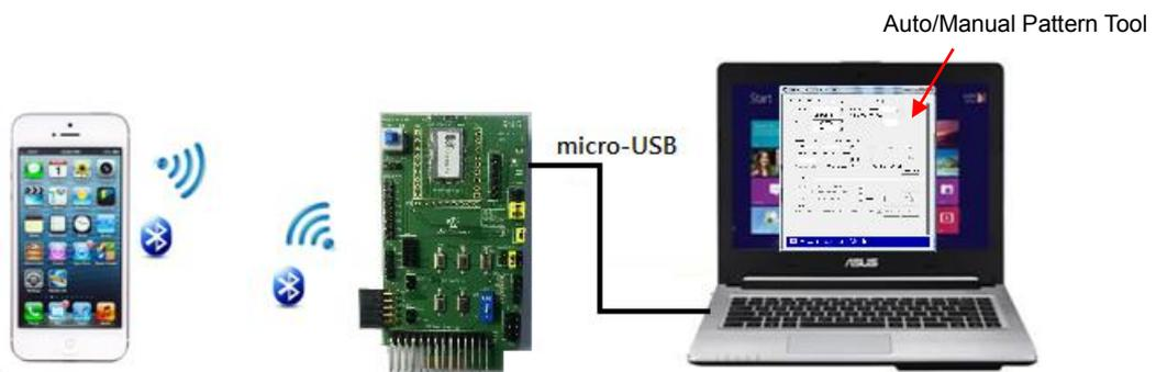
In the connection diagram, PC and the tool is acted as a MCU role to communicate with BM70 module by UART command set.
