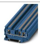
Feed-through terminal block, Connection method: Push-in connection, Cross section: 0.2 mm² - 6 mm², AWG: 24 - 10, Width: 6.2 mm, Color: blue, Mounting type: NS 35/7,5, NS 35/15
