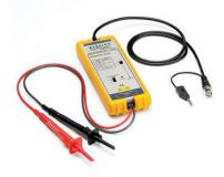
The TA041 is an active differential probe suitable for high common-mode voltage measurement applications up to  $\pm$ 700 V (DC + peak AC). It can be used with signal speeds of up to 25 MHz.
