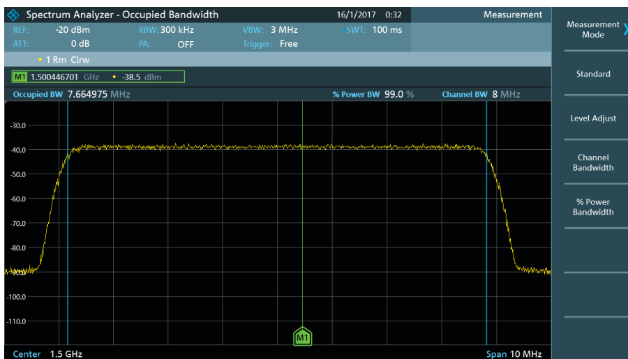
R&S®FPC-K55: occupied bandwidth.
