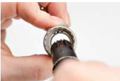
Step 14 - Push the sub- assembly into the shell
