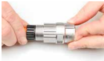
Step 15 - Push sub-assembly into shell
