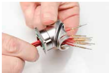
Step 4 - Crimp contacts onto wire
