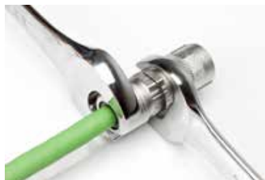
Step 16 - Tighten to 5-7 N/M using 25mm wrench
