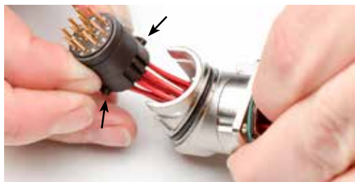
Step 5 - Locate keys on sides of insert
