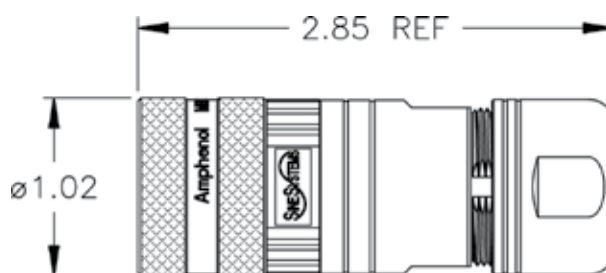
Plug kit straight, threaded; 7.5-11.0mm cord grip
