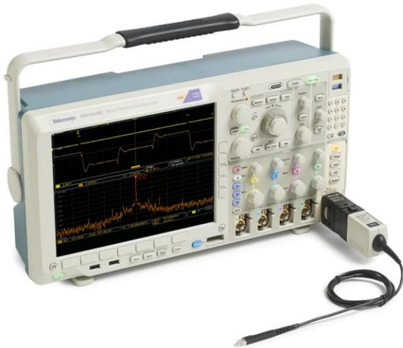
The optional TPA-N-VPI adapter enables any active, 50 Ω TekVPI probe to be connected to the RF input.
