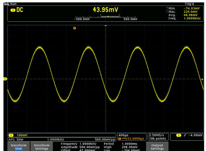
A DC measurement value is shown with a five second variation along with minimum, maximum, and average voltage values. The frequency of the waveform is also shown.
