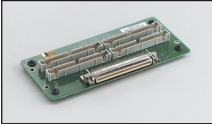
**CONN-3160-D1:** Screw Terminal Panel. The CONN-3160-D1 Adapter Panel brings all KPCI-3160 digital I/O signals out to an external panel via 50-pin headers. This panel allows connection of the ADP-5037 to allow the KPCI-3160 to operate the SRA-01 or ERA-01, ERB-24 or SSIO-24 relay products or to allow digital connections via the STP-50 or STA-50 Screw Terminal Panel and accessory boards. Requires the CAB-1800 or CAB-1800/S cable.
