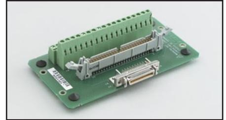
**STA-3108-D1:** Adapter panel that adapts the 36-pin connector (from the KPCI-3130 or KPCI-3132 digital I/O port) of the CAB-1284CC cable to a 50-pin header (mounted on the STA-3108-D1) with signals arranged for use with KPCI-PIO96 accessories.
