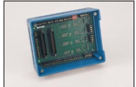
**STA-MB:** The STA-MB Screw Terminal Accessory provides sockets for 4 MB-Series modules. Two parallel 37-pin D male connectors provide interfaces for DAS boards and accessories. The MB-Series module inputs and outputs as well as the I/O connector pins are brought out to screw terminals. You then wire the MB-Series outputs to pins on the I/O connectors according to the requirements of your application.
