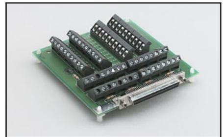
**STP-3140:** Screw Terminal Panel. Brings all KPCI-3140 signals out to external screw terminals. The STP-3140 comes with nylon standoffs, making it ideal for placing on a desktop or mounting in custom panels. Requires CAB-305 cable (1m/39").
