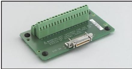
**STP-36:** Screw Terminal Panel. The STP-36 brings all KPCI-3130/3132, KPCI-PDISO8A, or KPCI-PIO32IOA signals out to external screw terminals. The standard versions come with rubber standoffs, making the STP-37 ideal for placing on a desktop or mounting in custom panels. Requires a CAB-1284CC-5 half-meter cable or CAB-1284CC-2 two-meter cable.
