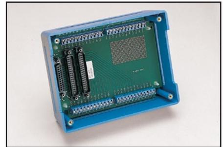
**STA-U:** The STA-U is a universal screw terminal accessory designed to connect to many Keithley data acquisition boards. It includes one 25-pin female D-type connector and two 37-pin male D-type connectors tied together. All 37 lines are brought out to screw terminal connections. A small breadboard area is available for additional circuitry. The STA-U is used for direct connec-
