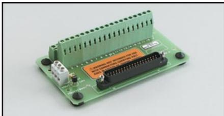
**STP-37:** Screw Terminal Panel with 37-pin male D-type connector and CJC sensor. The STP-37 is a cost-effective means of providing general-purpose screw terminal connections and CJC sensor. Requires a C1800 or S1800 cable.
