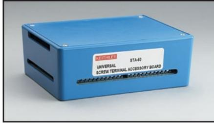
**STA-50:** The STA-50 is a universal 50-pin screw terminal board. Two 50-pin male connectors and a user breadboard area are provided. The signals on the two connectors are tied together and brought out to screw terminals. Requires a CACC-2000 cable.
