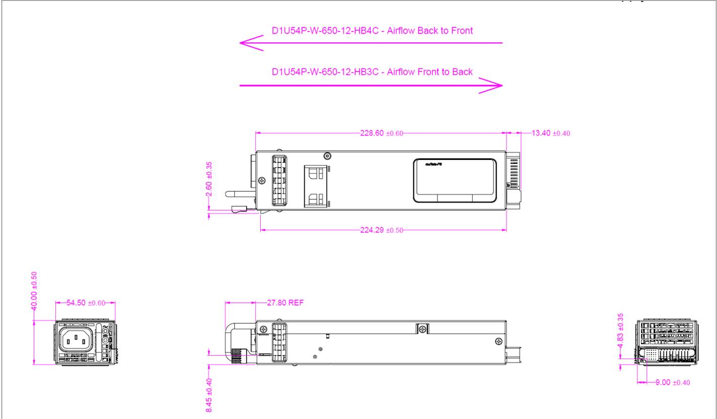
1. AC input connector: IEC 320-C14
