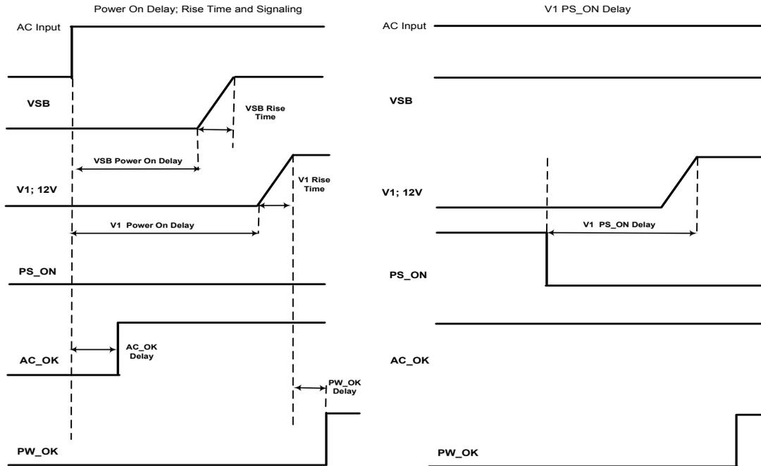
1. The turn-on delay after application of AC input within the operating range shall as defined in the following tables.
