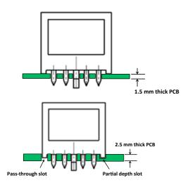
Note: The locking feature at the holder center must lock holder and PCB before welding.
