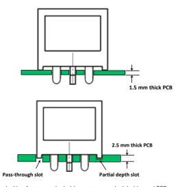
Note: The locking feature at the holder center must lock holder and PCB before welding.
