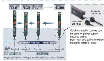
The sensors can be connected together with other sensors such as the FX-300 series of digital fiber sensors and the GA-311 of inductive proximity sensors. In addition, the SC series of sensor PLC connection units with MIL connector compatibility can also be used to further reduce the amount of wiring.
