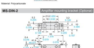
Material: Cold rolled carbon steel (SPCC) (Uni-chrome plated)
