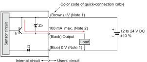
Notes: 1) The quick-connection sub cable does not have +V (brown) and 0 V (blue). The power is supplied from the connector of the main cable.
