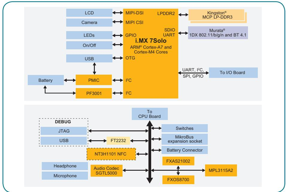
Another key component in the platform is a multi-chip memory module with 8 GB of managed NAND with eMMC 5.0 interface for storage and 4 GB LP-DDR3 for application code. Its compact size and low power make it ideal for IoT and wearable devices.
