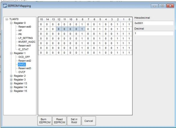
Note: To program the EEPROM, you have to provide a 20.6V voltage supply to the "P" contact (GND reference has to be connected with the GND contact):
