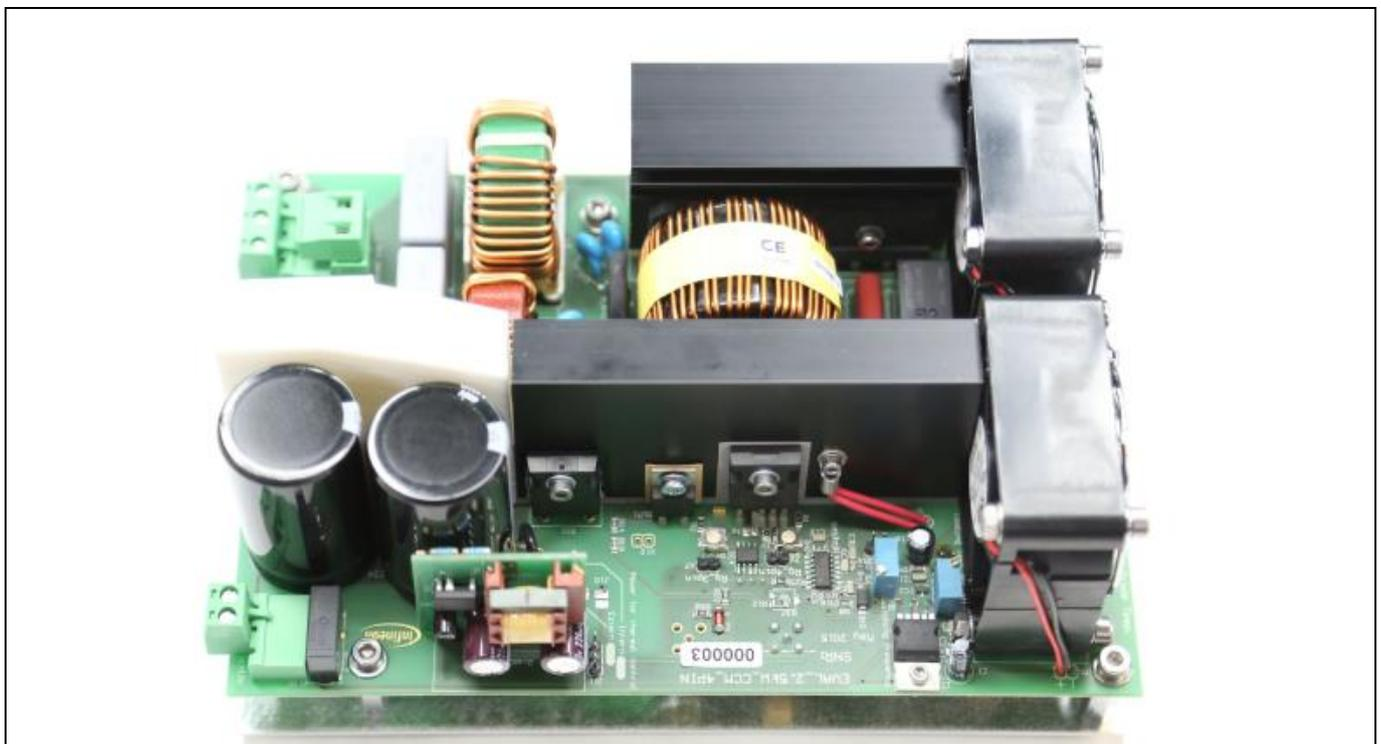
Figure 2 EVAL\_2.5kW\_CCM\_4PIN evaluation board
