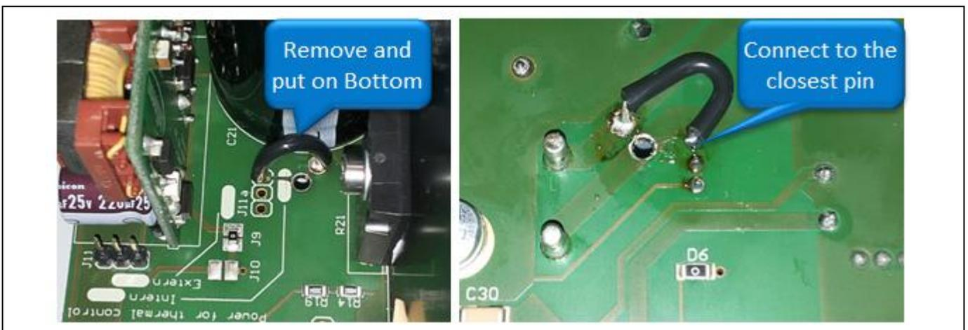
Figure 3 Wire change from top layer to bottom layer
