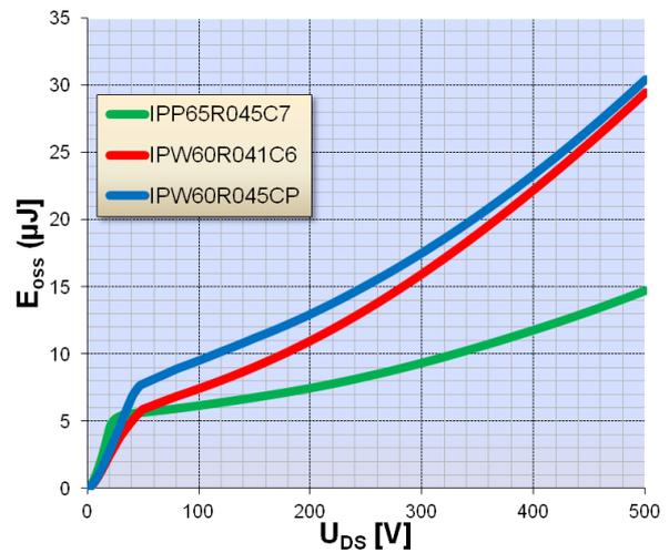
Figure 7:  $E_{oss}$  as a function of  $V_{DS}$  for C6, CP, and C7 CoolMOS™ in the  $R_{DS(on)}$  class of 41–45m $\Omega$ .
