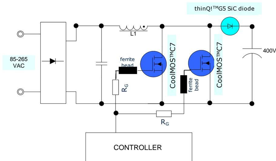
**Figure 36: Schematic of parallel MOS operation with ferrite bead on the gate**
