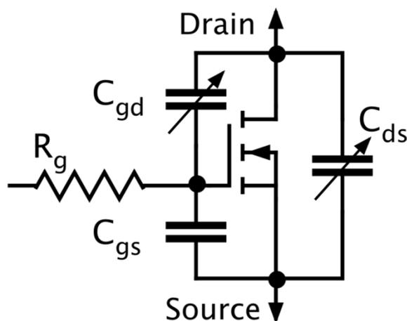
Figure 14: Basic elements controlling MOSFET switching
