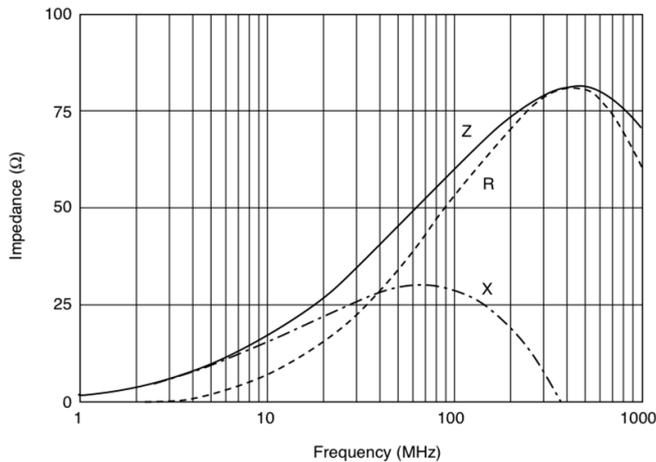
**Figure 35: Impedance-frequency characteristics of BLM41PG600SN1 ferrite bead**
