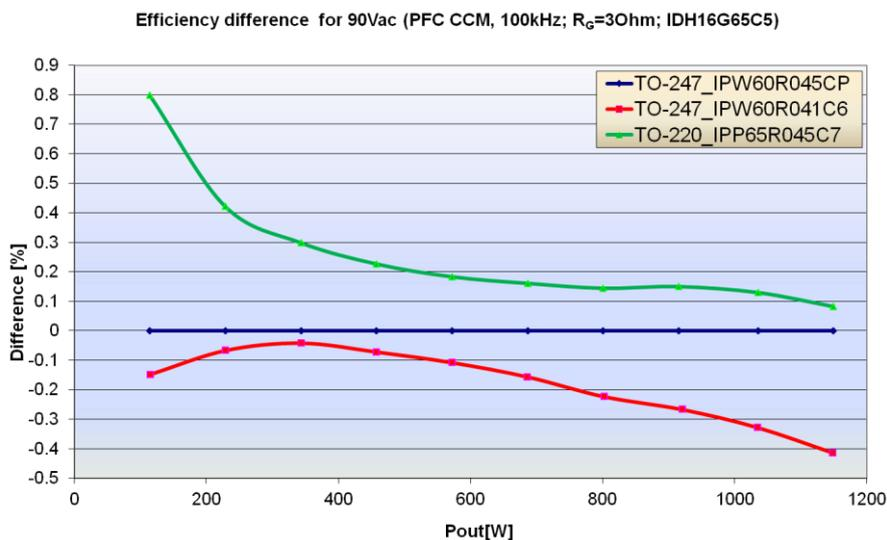
**Figure 13: Efficiency comparison of IPW60R045CP, IPW60R041C6, and IPP65R045C7**
