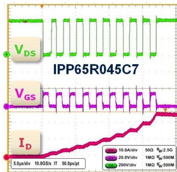
**Figure 32: Gate ringing test with IPP65R045C7 for current stepped up to 25A for  $R_G=3\Omega$**
