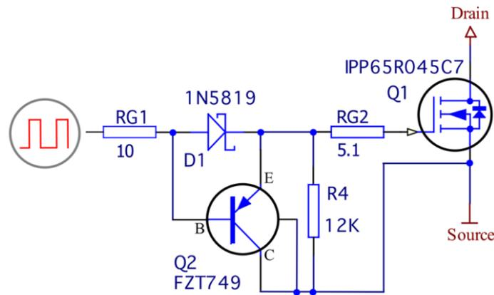
Figure 27: PNP pull down gate drive
