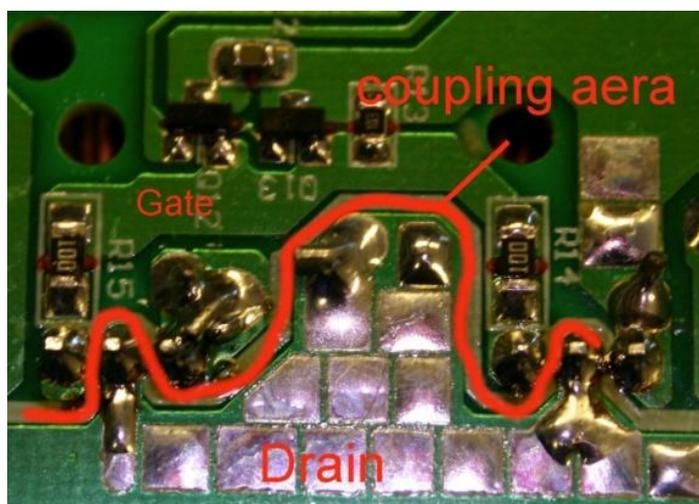
**Figure 26: Commercial layout leading to problems due to close proximity of gate and drain**
