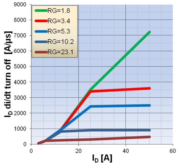
Figure 21: CP turn-off di/dt for  $V_{GS}=12V$  as a function of drain current for  $R_G = 1.8 - 23\Omega$
