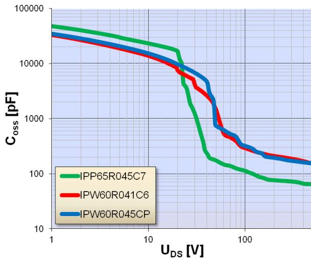
Figure 6:  $C_{oss}$  as a function of  $V_{DS}$  for C6, CP, and C7 CoolMOS™ in the  $R_{DS(on)}$  class of 41–45m $\Omega$ .
