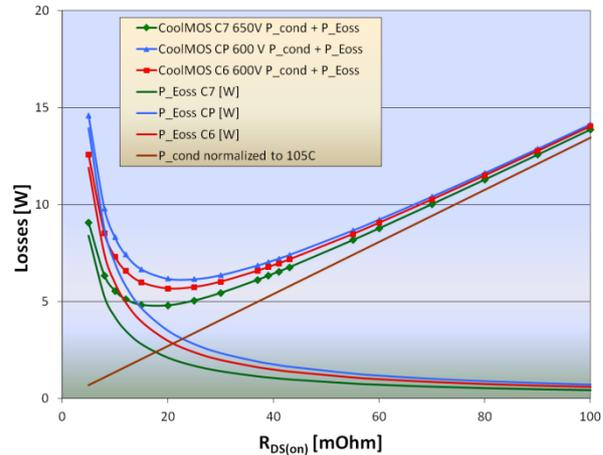
Figure 11:  $E_{oss}$  vs.  $R_{DS(on)}$  loss balance 800W PFC at 70 kHz for 90VAC input
