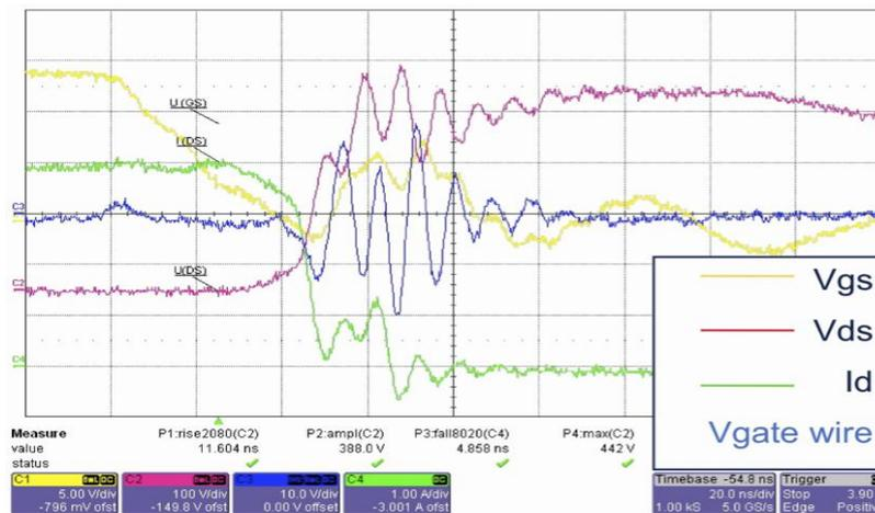
Figure 28: Turn-off waveforms with gate oscillations arising due to interaction in the gate to source circuit during turn-off
