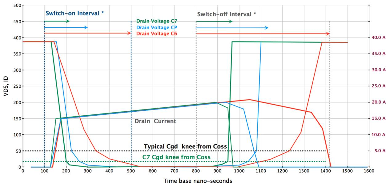
**Figure 17: Switching simulation comparison for  $V_{DS}$  and  $I_D$**
