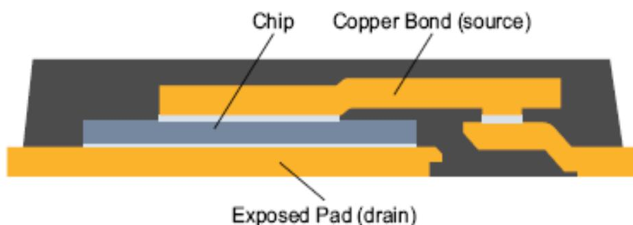
Figure 3 Cross section showing construction of a clip bond (e.g. TDSON)
