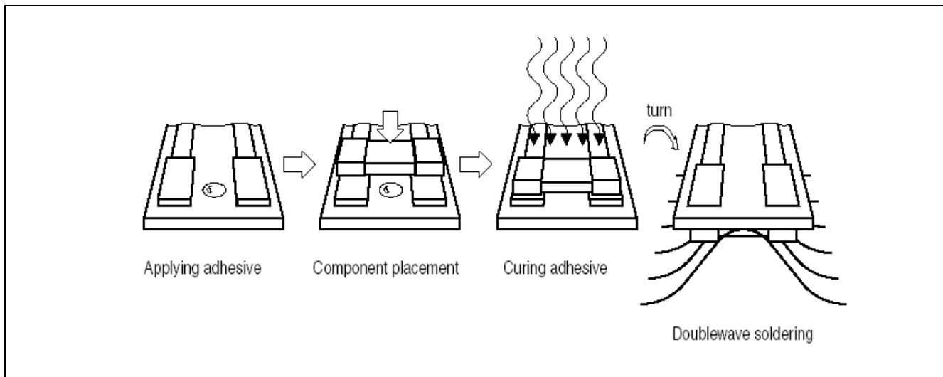
**Figure 9 Attachment of SMD devices prior to wave soldering**
