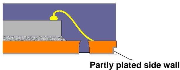
**Figure 5 Schematic cross section of a LTI (lead tip inspection) feature**
