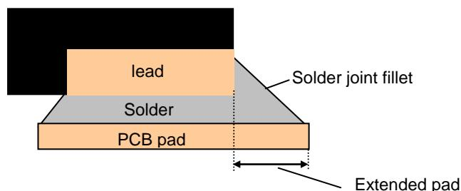
**Figure 7 Schematic cross section of a perimeter lead**
