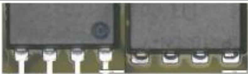
**Figure 12 Typical optical photos of SuperSO8 solder joints. Those of gate and source can be seen on the left side. The right side shows the four soldered extensions of the big drain pad.**
