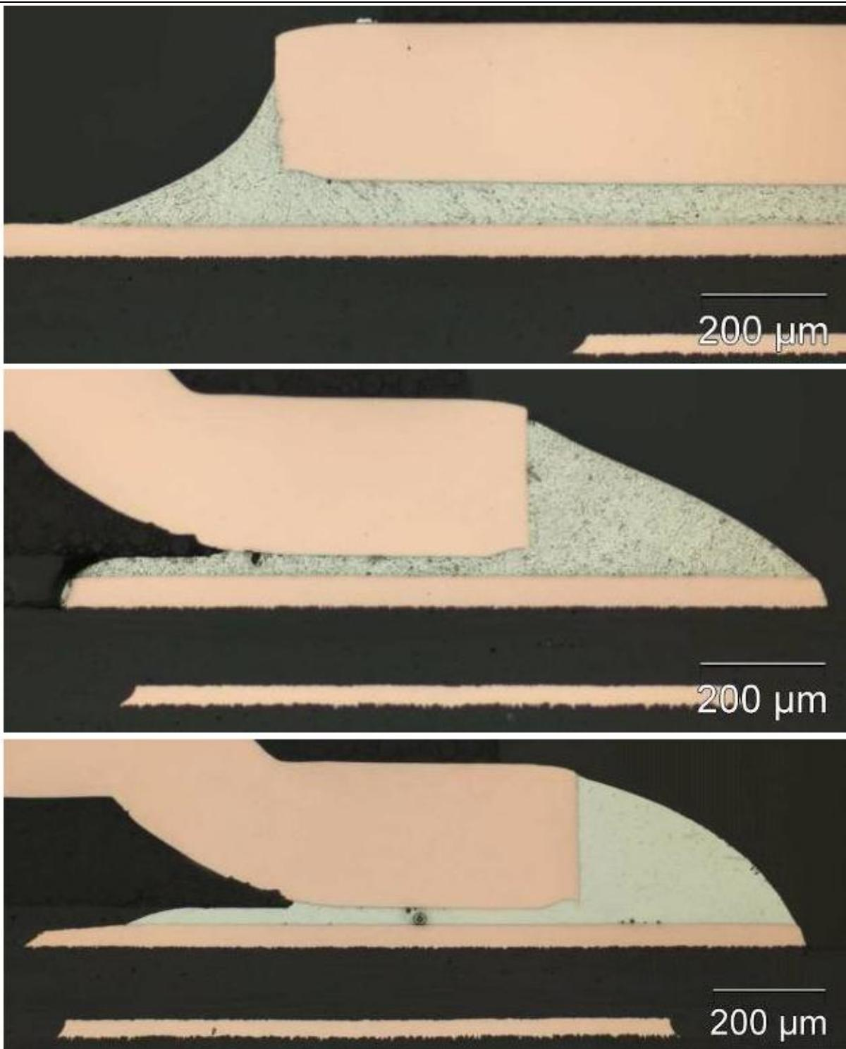
**Figure 14** Cross-section views of mounted TDSon-8 packages. The first photo shows a SnPb solder joint of the drain pad. The second and third photos show source/gate solder joints with SnPb, and SnAgCu alloys, respectively.
