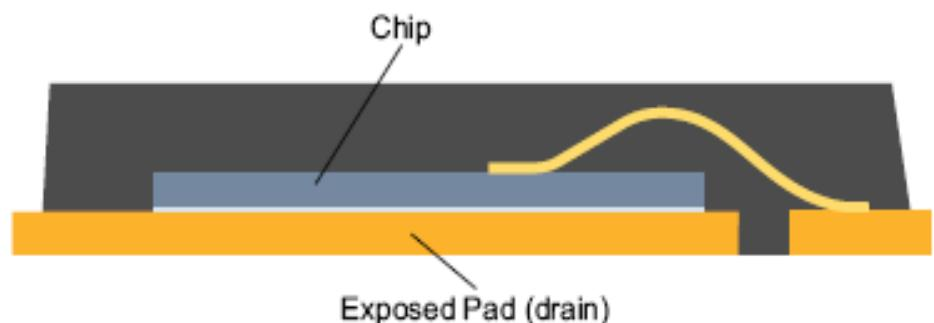
Figure 2 Cross section showing construction of a wire bond (e.g. TDSON)
