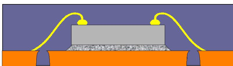
Figure 4 Cross section showing construction of a two-sided wire bond package (e.g. USON)
