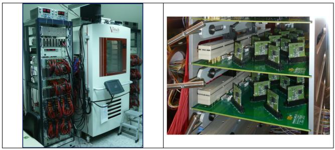
Figure 4 Test bench for repetitive avalanche
