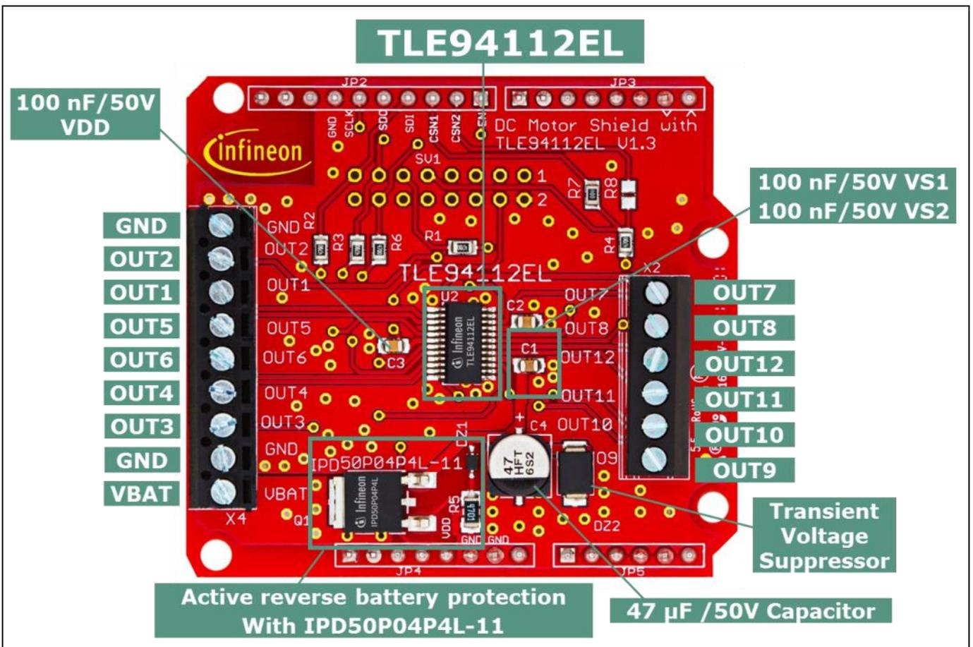
Figure 1 DC Motor Shield with TLE94112EL
