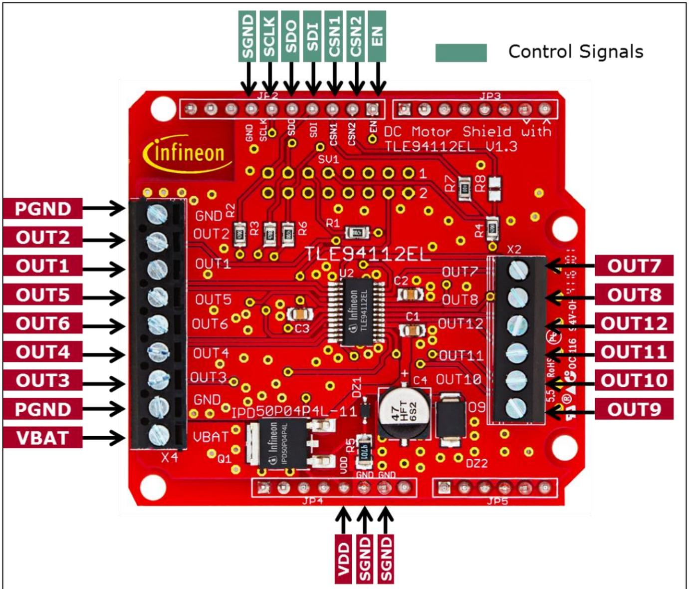
Figure 3 DC Motor Control Shield connectors
