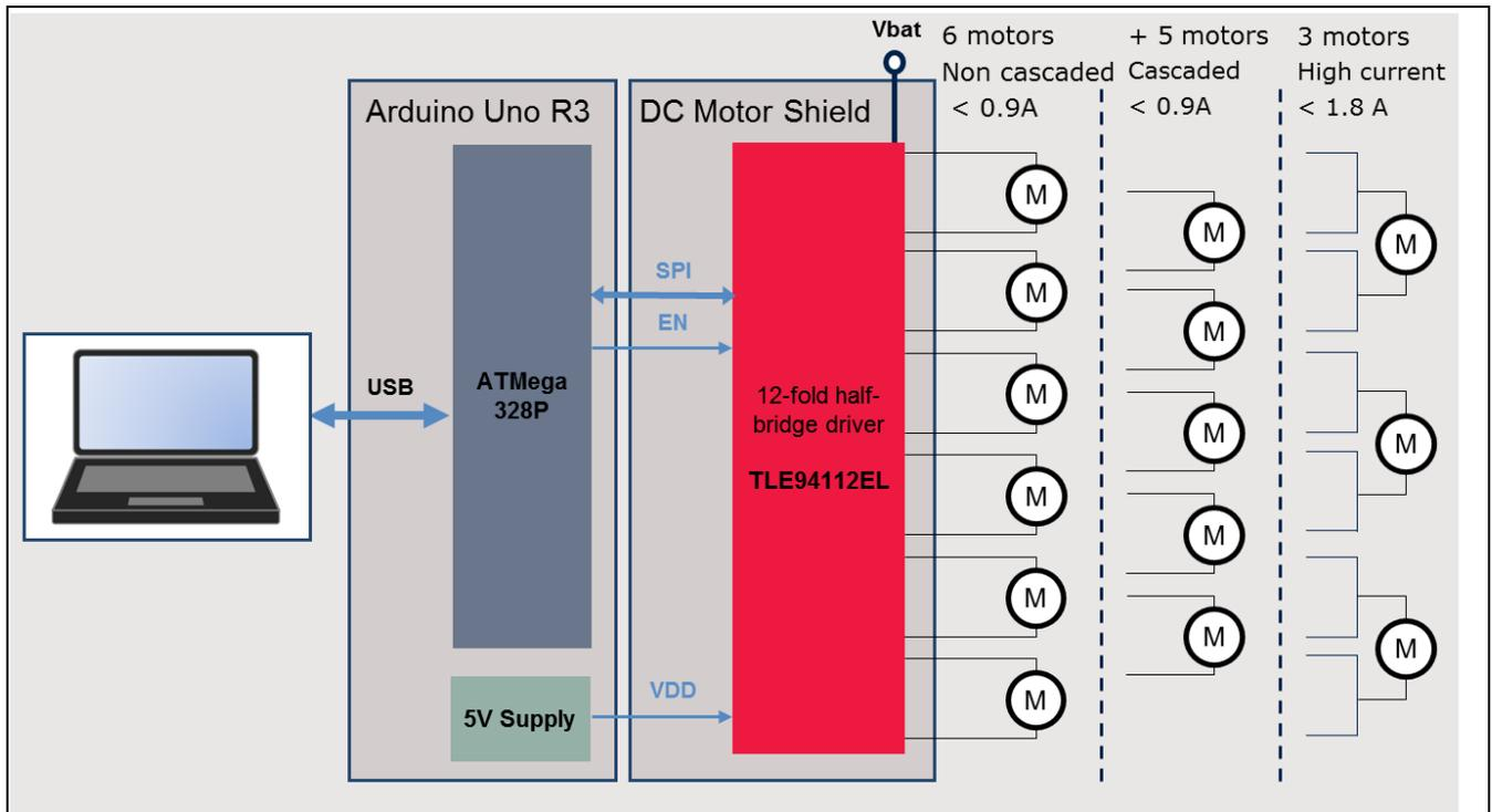
Figure 2 Simplified application diagram with TLE94112EL driving DC motors
