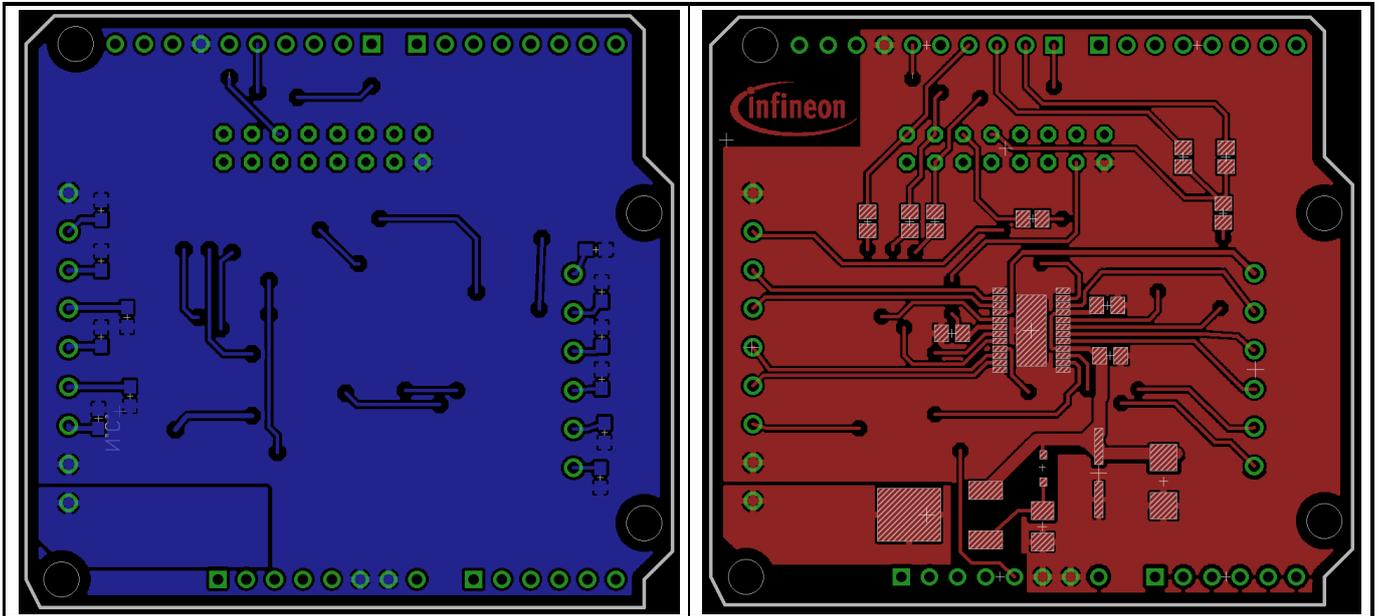
Figure 2 Figure 5 DC Motor Control Shield – Bottom and top layers
