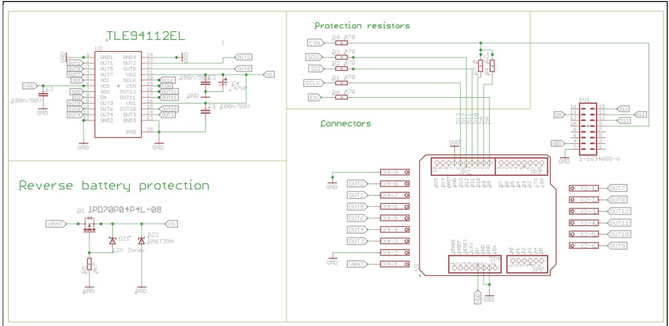
Figure 1 Figure 4 Schematics Motor Control Shield for Arduino with TLE94112EL
