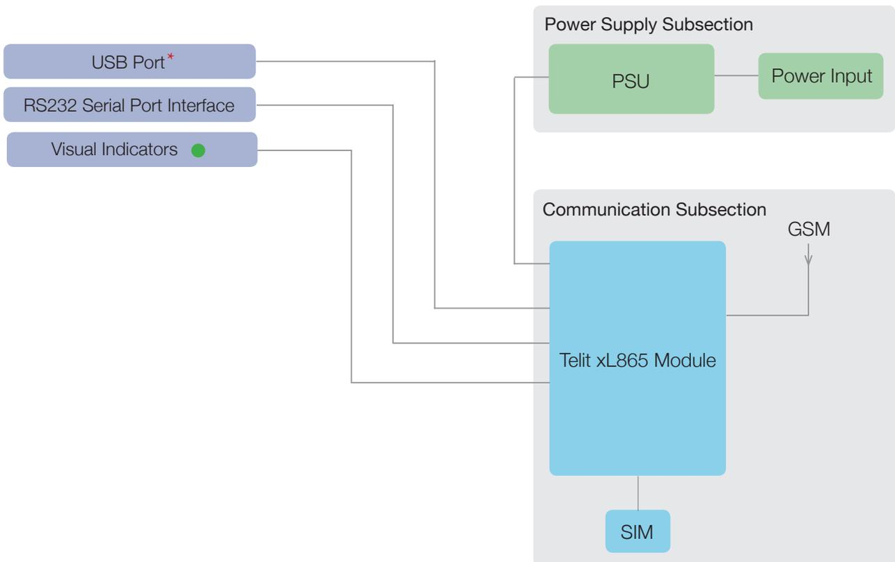
\* USB interface only provides power for LC200-GPRS and provides serial data and power for LC200-UMTS.
