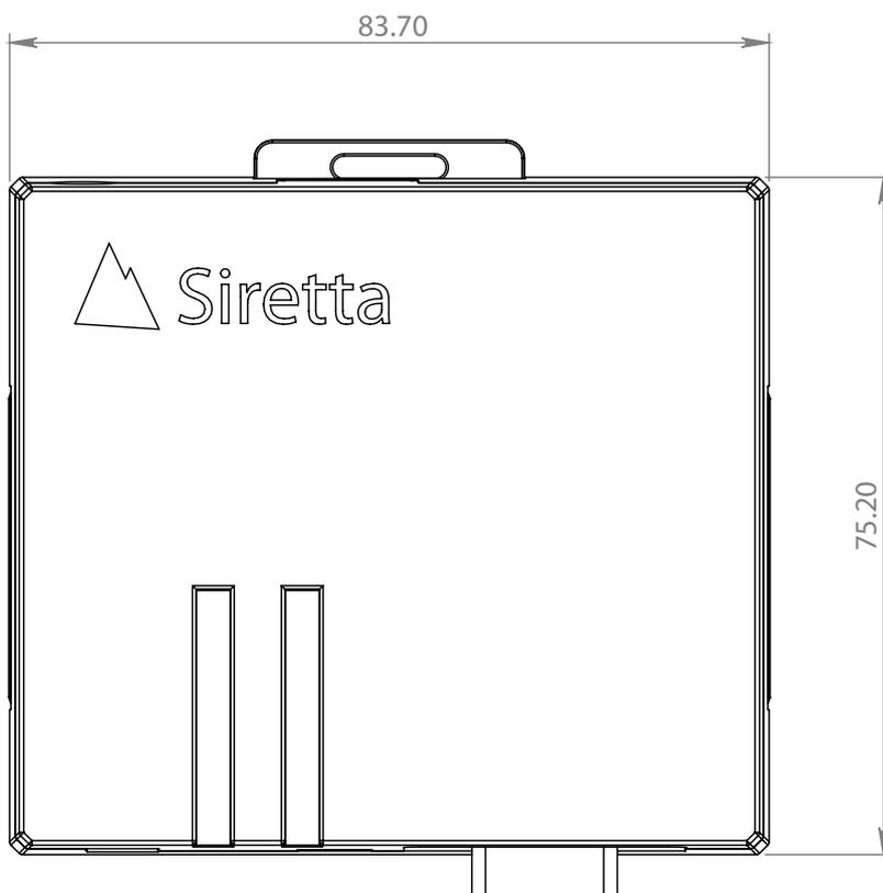
Figure 3. LC200 modem side view - dimensions
