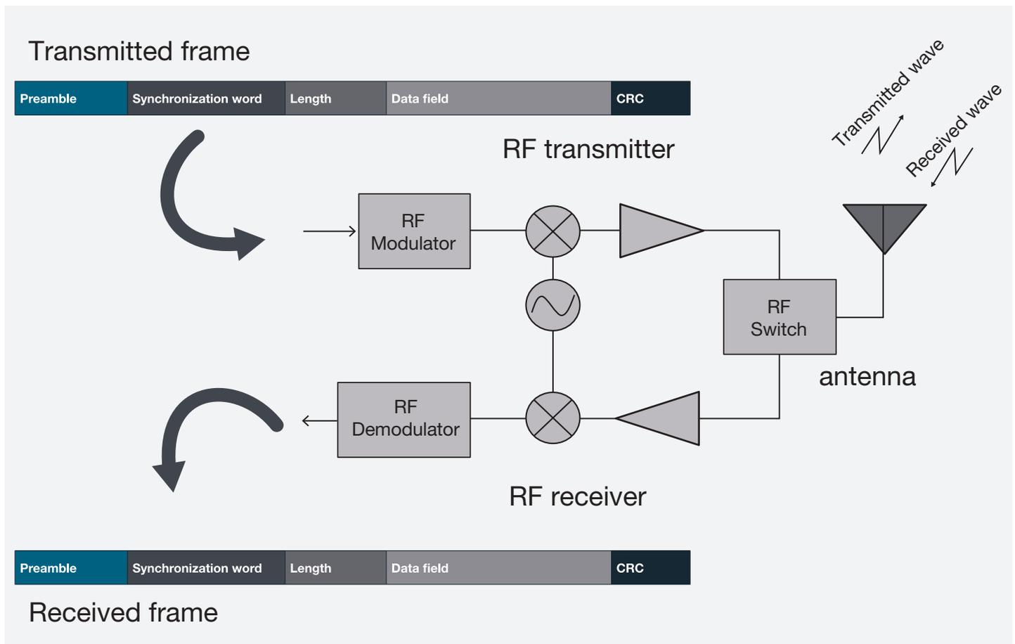
**Figure 5.** A diagram of the main components of the radio transceiver system.
